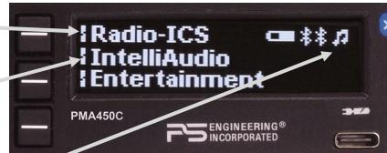
A **split bar** on a line indicates that a *secondary* function is available when that button is held for more than 1 second. For example, on the home screen, this function is:
