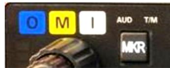
The Marker receiver is always on. Push the **"MKR"** button to hear the tones. **AUD** will light up green when the marker audio is on.
